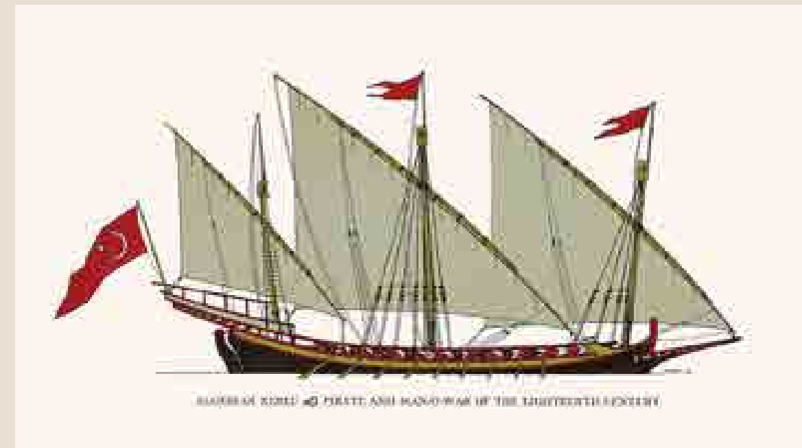
The xebec was a lightly-constructed vessel that featured lateen sails as well as oars. It was considered as an elusive ship that in the expert hands of Barbary corsairs 'arose, raided, and disappeared' – Hugh Evelyn Prints
