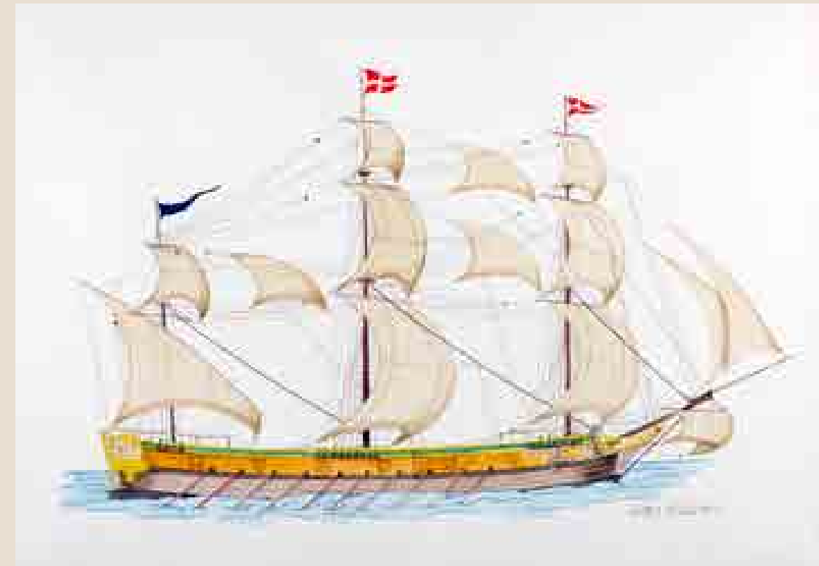
A corvette was a small and fast naval vessel ranking in size below a frigate. In the 18 th century corvettes were three-masted ships with square rigging similar to that of frigates and ships-of-the-line, but they carried only about 20 guns on the top deck. The Santa Teresa and the San Francesco di Paola were the first two corvettes of the Order – Courtesy MMM
